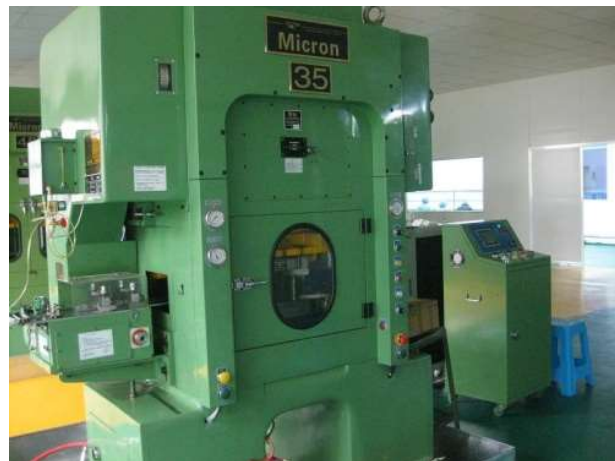
35 Tonnage High Precision Stamping Machine
